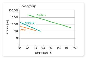
Arnitel C stands out due to its successful testing at a continuous use temperature of 175°C for 3,000 hours, all while maintaining its flexibility and strength better than polyamide 12 (PA12) which tends to embrittle under these conditions.
